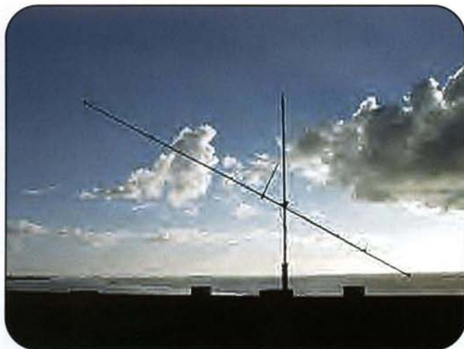
Seven-element long-boom Yagi at KH0/KH2K. (Photo courtesy of JA1RJU)
