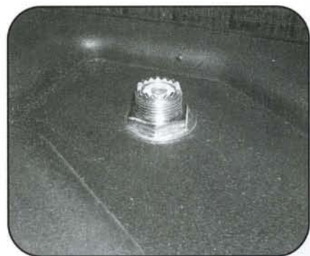
Photo 5. A feedthrough connection on the top of the box provides a place to connect VHF antennas.
