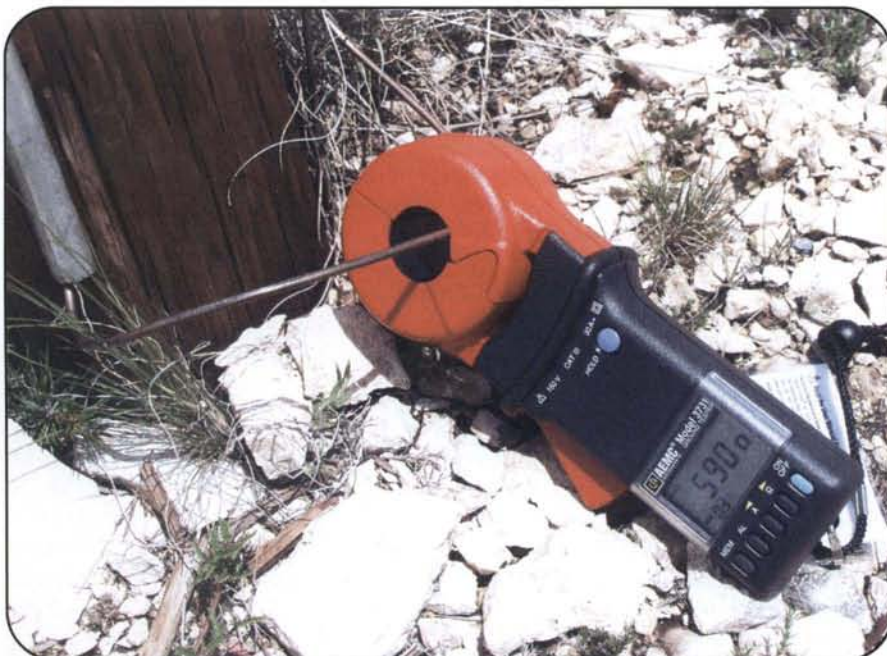
Photo 5B. Direct clamp-on measurement of the utility pole ground-wire resistance—590 ohms.
