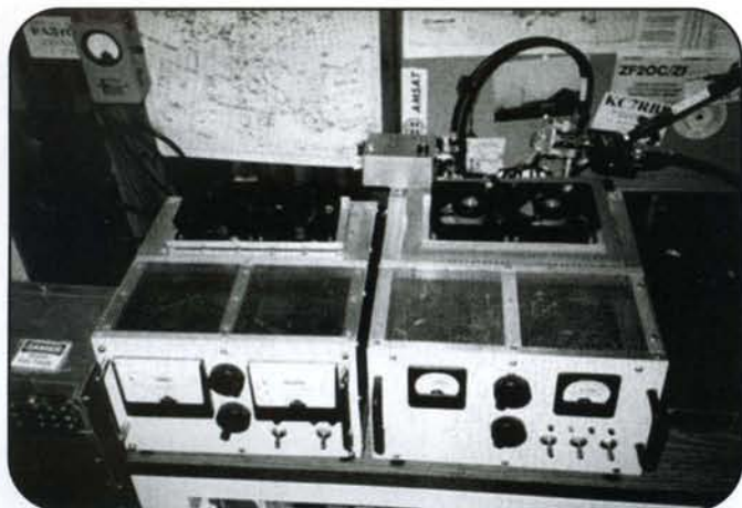
Addition of fans to reduce blower back pressure on W7GJ's amplifiers.
