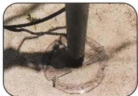
Mast bracing and antenna rotating is most easily accomplished with a single yagi. If the azimuth and readout are manual, you can bury the mast in the ground (resting upon a solid object such as a board or concrete block), with a protractor around the mast. An indicator such as a bent paper clip taped to the mast is a very accurate and simple indication of direction.
