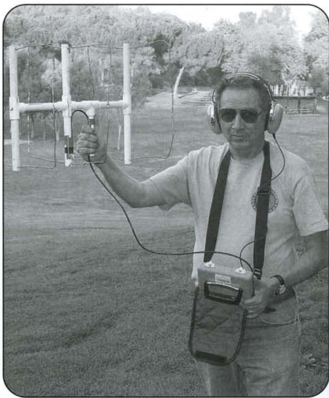
For tracking 216-MHz pulsed radio tags in Project Lifesaver, Sam Vigil, WA6NGH, uses a three-element stiff-wire quad scaled from a 2-meter design.
