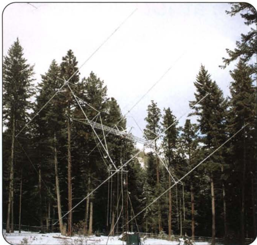
Six-meter EME array at W7GJ ( 4 \times M^2 6M9KHW fed with 1\frac{5}{8} -inch heliax).
