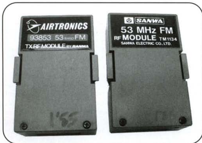
Airtronics 6-meter transmitter modules which plug into the back of the company's transmitters.
