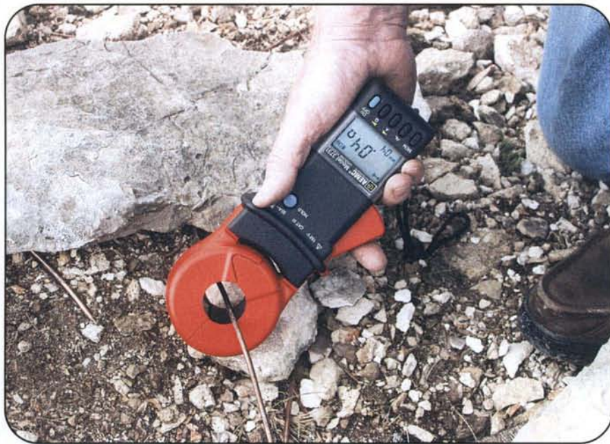
Photo 5A. Direct clamp-on measurement of the ground conductor resistance near the radio shack. Unit reads less than 0.1 ohm, its limit of resolution.
