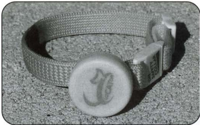
This LoCATor pet tag weighs one-half ounce and has a break-away link to prevent accidental choking of the animal. (All photos by Joe Moell, KØOV)
